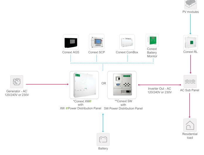
XW+ Single-phase or split-phase (120/240VAC or 230 VAC) solution with optional AGS/Generator (7.0 kW - 25.5 kW) \*Up to two slave units are optional to increase power
